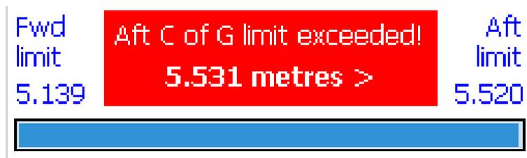
In this situation, the Aft C of G limit has been exceeded and is indicated by the arrow > and the blue bar which is fully over to the right. In this situation you can either add pilot row ballast (on
